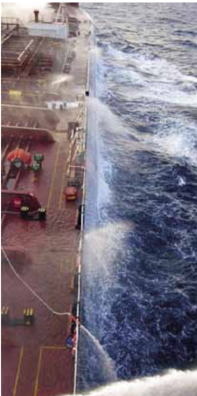
Water sprays and waterfalls are some of the measures used to avoid pirates boarding the vessel.
